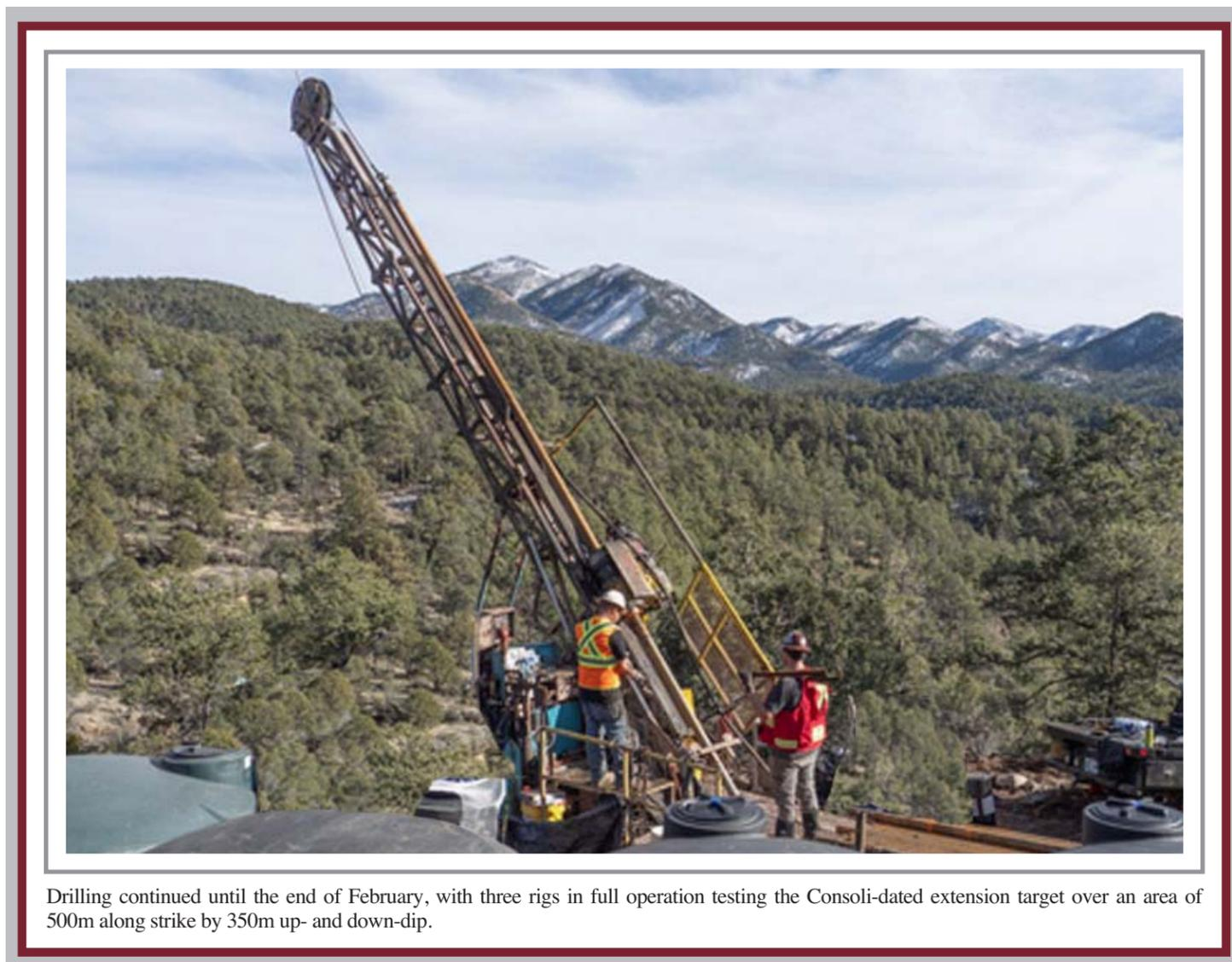
Drilling continued until the end of February, with three rigs in full operation testing the Consolidated extension target over an area of 500m along strike by 350m up- and down-dip.
